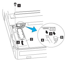
Where: A is the IR Cable. B is the Standby Battery Cable. C is the IR Lens.
